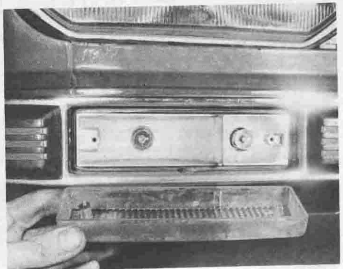
23.1 Removing the front parking and flasher lens
