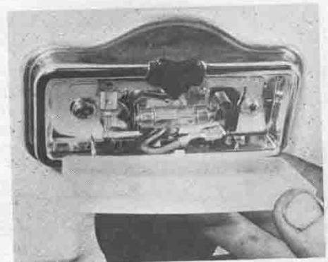
27.1 Removing the courtesy lamp lens to change a bulb
