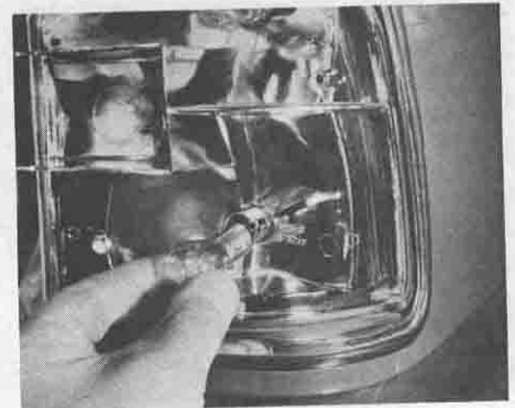
25.3 Fitting a new tail lamp bulb
