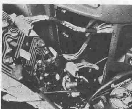
34.2 With the panel pulled out the bulbs can be reached
