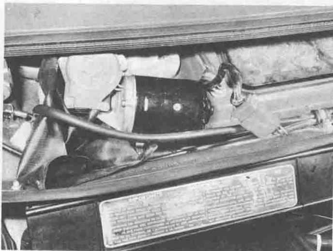
51.4 The wiper motor is mounted in the channel section between the scuttle and engine bay
