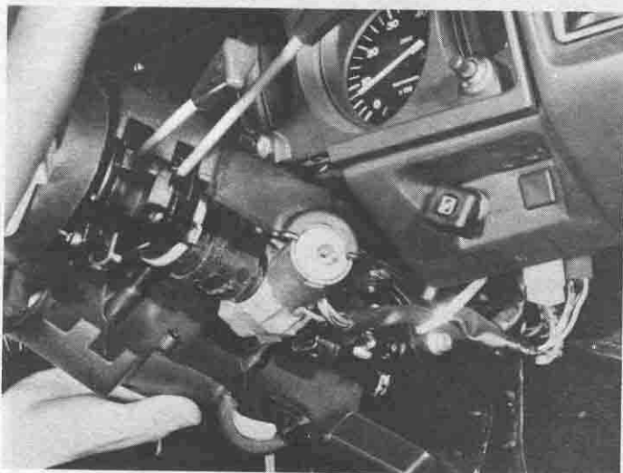
36.4 Removing the steering column lower casing
